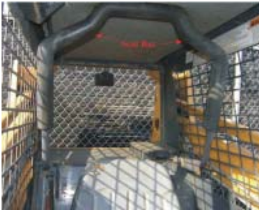
Figure 2: Typical Control Interlock System (seat bar, shown in raised position)
